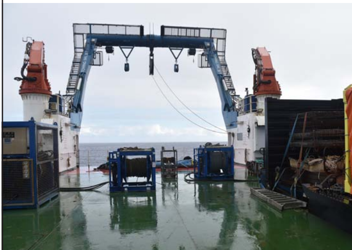
View from the main working hangar looking aft to the A-frame which is used during surveys to deploy the net used for collecting specimens at various depths in the ocean.
