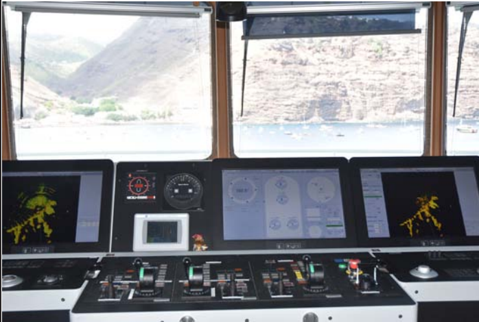
The high-tech Bridge or Wheelhouse – the ‘brain’ of the Ship.....there is not a steering wheel in sight as most controls are with joystick features.
