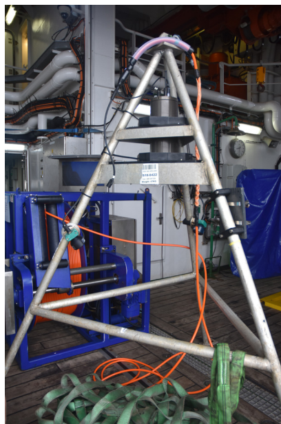
Tripod used for supporting underwater camera on the sea-bed
