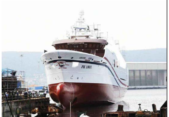
Argos Cies is 75 metres long, has 1,998 gross tonnage and will carry up to 50 crew members. She will be delivered by Nodosa shipyard at a cost of €21 million
