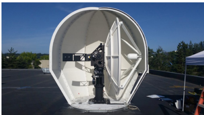
An example of a small satellite tracking station; this one appears to be on a roof top
