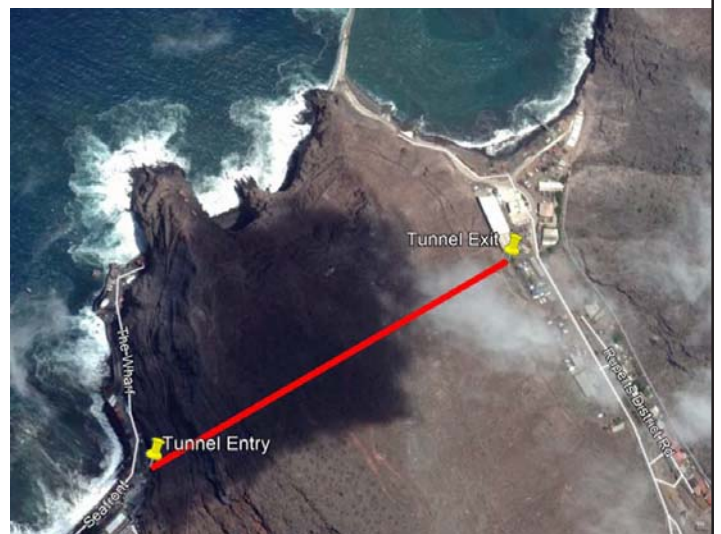
One of three routes considered for a tunnel linking Rupert's and James Valleys. Estimate for a single carriageway width is £8 – 10 million or £14.5 million for double width
