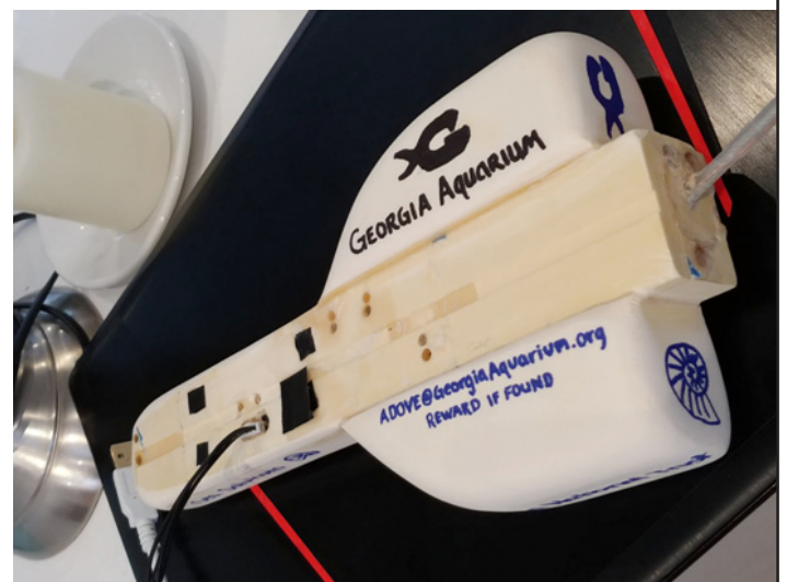
A custom deep hardened satellite tag developed as a collaboration between Georgia Aquarium and iSea Solutions principal engineer Thom Maughan, with funding from SHNT and Blue Marine Foundation. Pic: Al Dove
